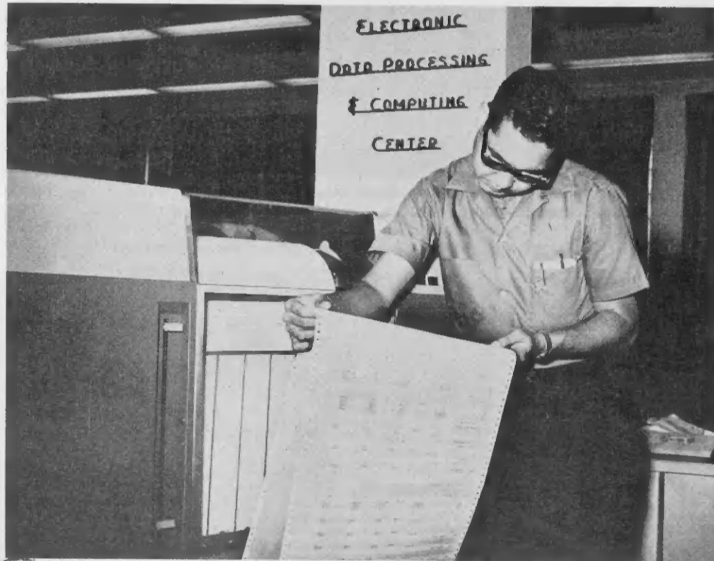
THE PRINTER can be loaded with paper in a matter of seconds. Since skipping between the printed lines is up to sixty times as fast as printing, faster document output can be obtained than just from printing speed alone.
